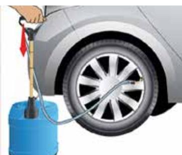
Switch off the valve tap and remove pump from valve.
